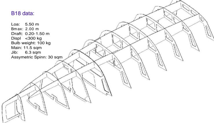
Backman 18 can be built by you or a local boatbuilder from precut kits. All parts are precision cut on a cnc laser ready for a quick assembly.
